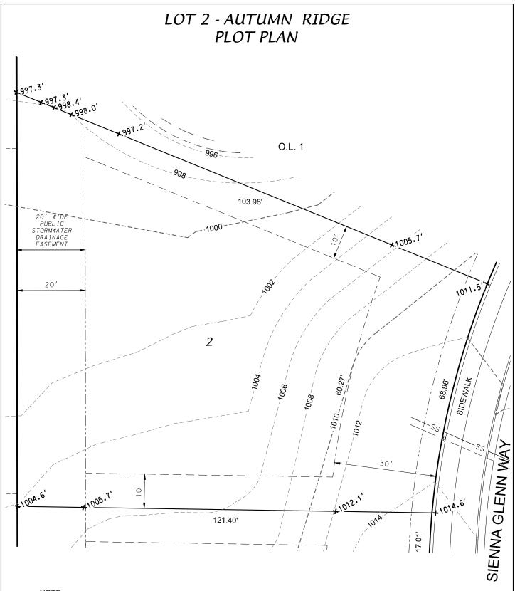
NOTE: MINIMUM ELEVATION OF TOP OF FOUNDATION WALL = 998.8
