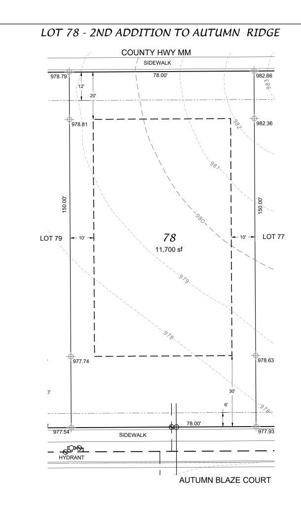
NOTE: MINIMUM ELEVATION OF TOP OF FOUNDATION WALL = 978.5
