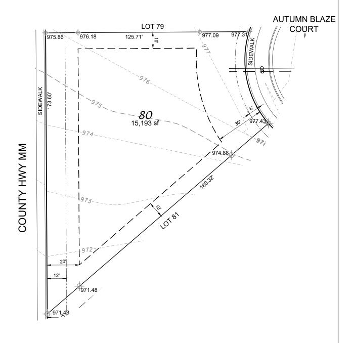
NOTE: MINIMUM ELEVATION OF TOP OF FOUNDATION WALL = 972.3
