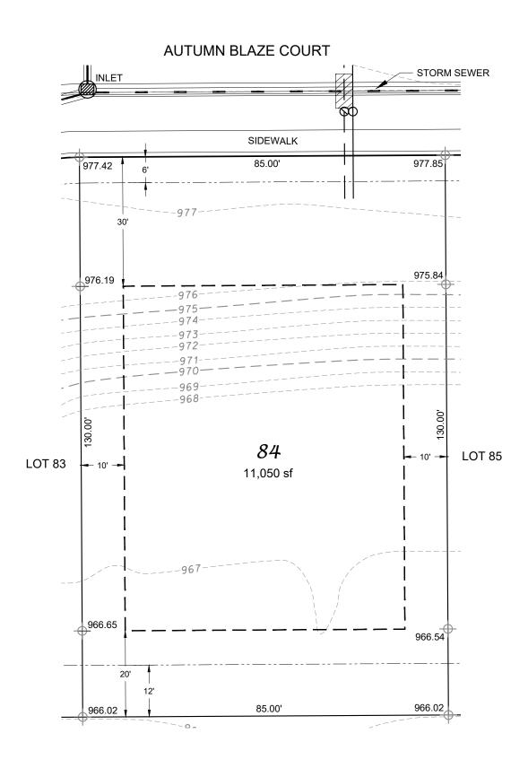
NOTE: MINIMUM ELEVATION OF TOP OF FOUNDATION WALL = 969.5
