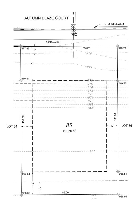
NOTE: MINIMUM ELEVATION OF TOP OF FOUNDATION WALL = 968.0
