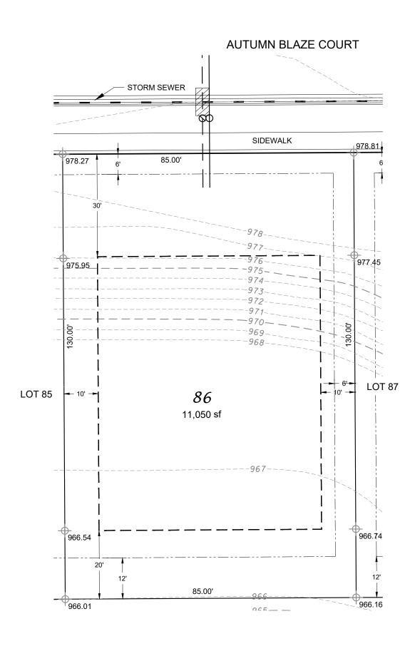
NOTE: MINIMUM ELEVATION OF TOP OF FOUNDATION WALL = 968.5
