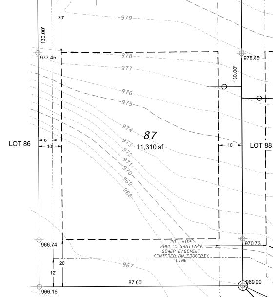
NOTE: MINIMUM ELEVATION OF TOP OF FOUNDATION WALL = 967.5
